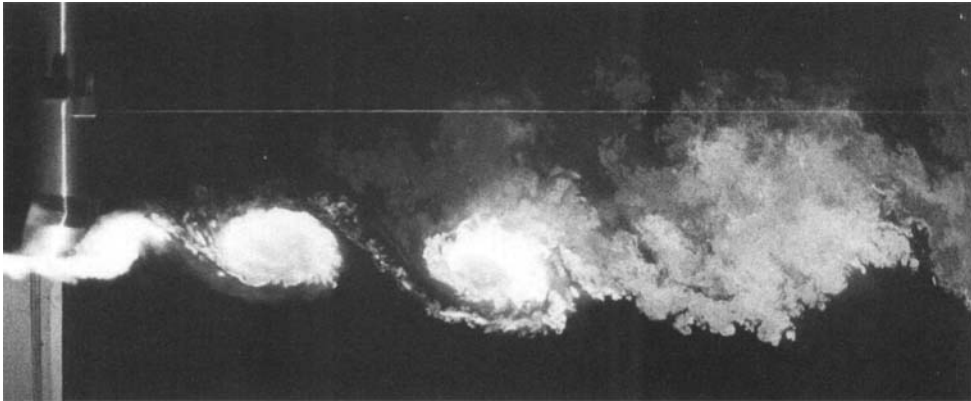
FIGURE 10. Flow development at strong excitation and clean separation showing sudden diffusion and vortex breakup.
